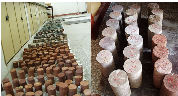
Fig. 10 Rock specimens from three shaft inspection holes of the Ying-Pan-Hao coal mine
