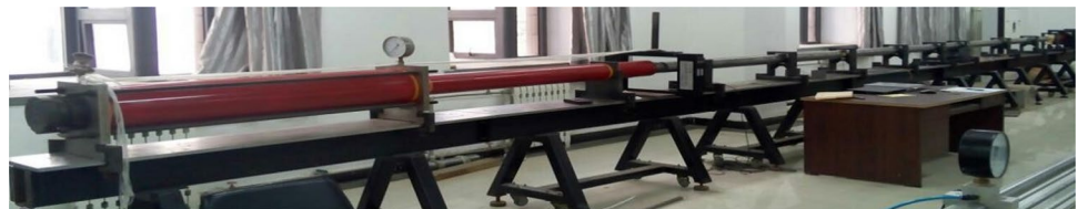
Fig. 4 Split Hopkinson pressure bars (SHPB) equipment
