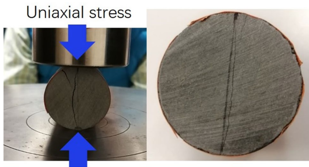
Fig. 2 Photograph of a Brazilian test (left) and the resulting diametral macro-crack (right)
