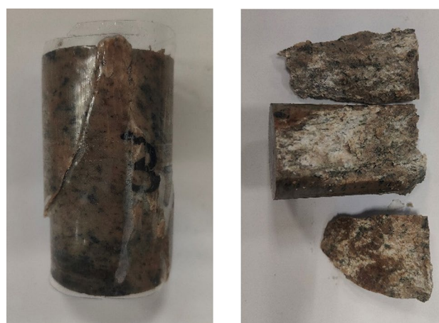
Fig. 16 Fatigue failure of specimen 3–1
