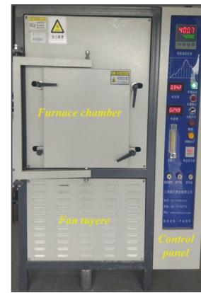
(a) High-temperature treatment equipment
