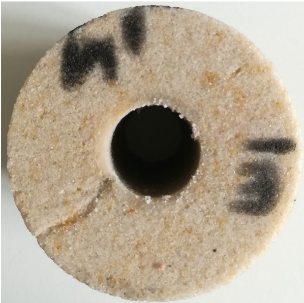
Fig. 9 View of BS8, cut at the middle point. A clear non-planar, arcuate fracture is present on the SW quadrant as well as a minor, barely visible fracture on the NE quadrant (visible around halfway between the borehole and the edge of the sample)
