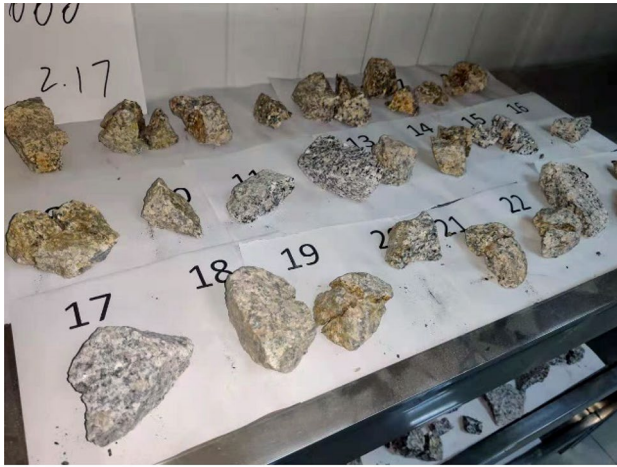
Fig. 4 Typical point load strength test specimens
