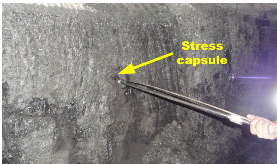
Fig. 19 a Coal pillar of underground coal mines at 3 and 4 incline mine, Jhanjra, b installation of stress capsule in the coal pillar of 3 and 4 incline mine, Jhanjra
