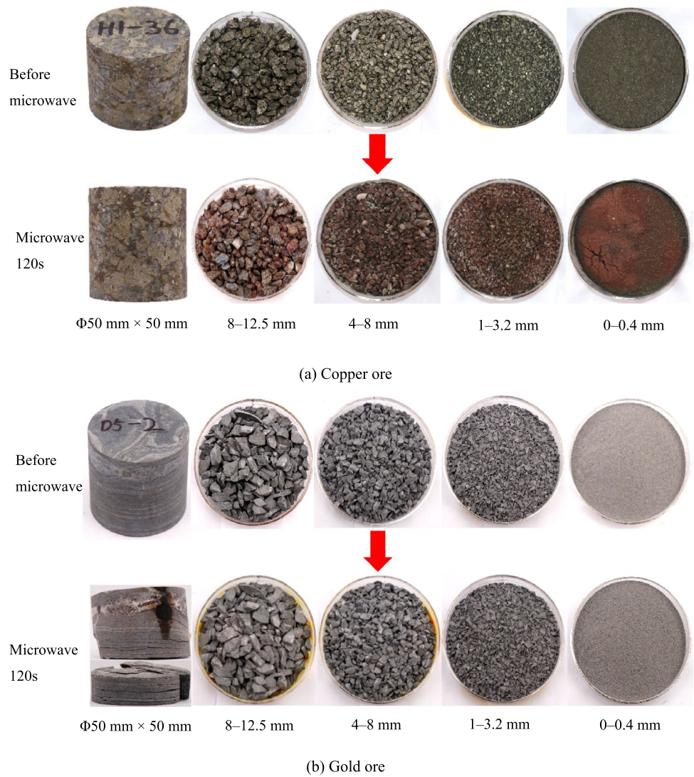
Fig. 6 Photographs of the ore samples before and after microwave heating
