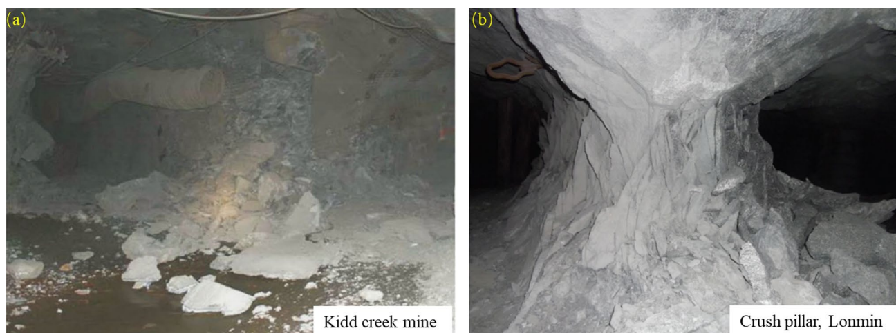
Fig. 1 Photographs of a rock burst at the cross point of roadway of Kidd Creek mine (Cai and Kaiser 2018) and b crush pillar of Lonmin (Plessis et al. 2014)
