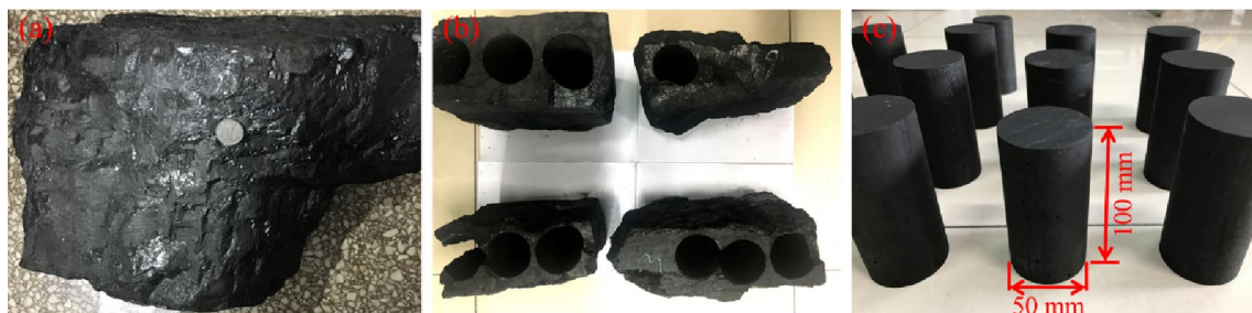
Fig. 1 Necessary information on experimental material: a one of the original coal blocks sourced from the coal mine; b coal blocks after being cored; c standard intact coal samples without macroscopic bedding planes
