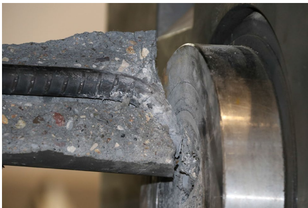
Fig. 8 Failure pattern of rock bolt subjected to shear load
