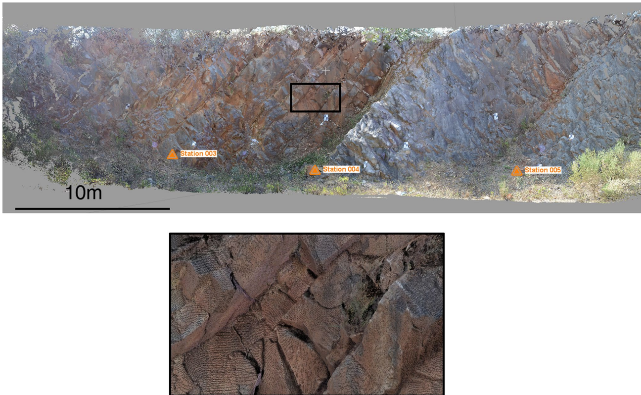
Fig. 9 TLS point cloud representing the whole slope under study (top); the three different scan positions are highlighted (triangles). Details of the point cloud (bottom)
