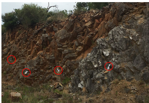
Fig. 6 Example of targets measured during the topographic survey for the UAV flights and TLS alignment and georeferencing
