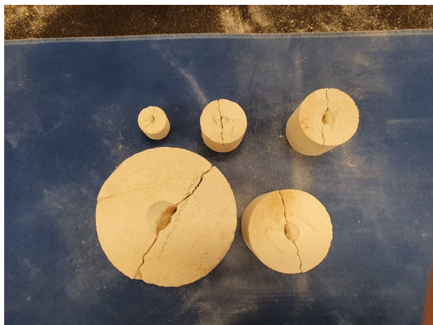
Fig. 18 Typical failure patterns observed from the axial point load tests on Gambier limestone
