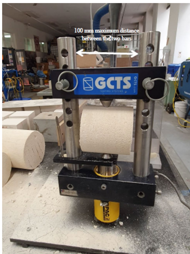
Fig. 7 GCTS point load testing frame used for the point load experiments. The arrow indicates the limitation of frame where the sample larger than 100 mm diameter could not be tested
