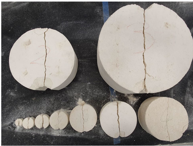
Fig. 15 Typical failure patterns observed from the Brazilian tests on Gambier limestone
