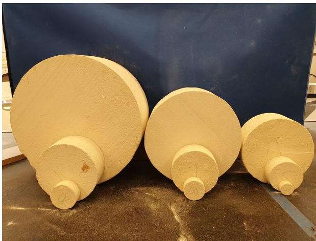
Fig. 3 Examples of Gambier limestone samples with different sizes for Brazilian test
