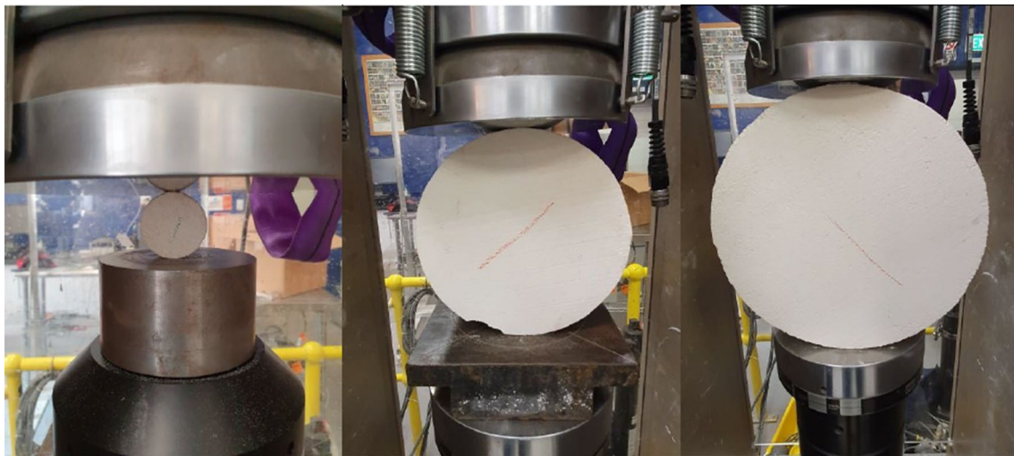
Fig. 6 Examples of different Brazilian testing setups for the samples with various sizes
