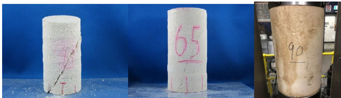
Fig. 13 Typical failure patterns observed from the uniaxial compressive tests on Gambier limestone with different diameters
