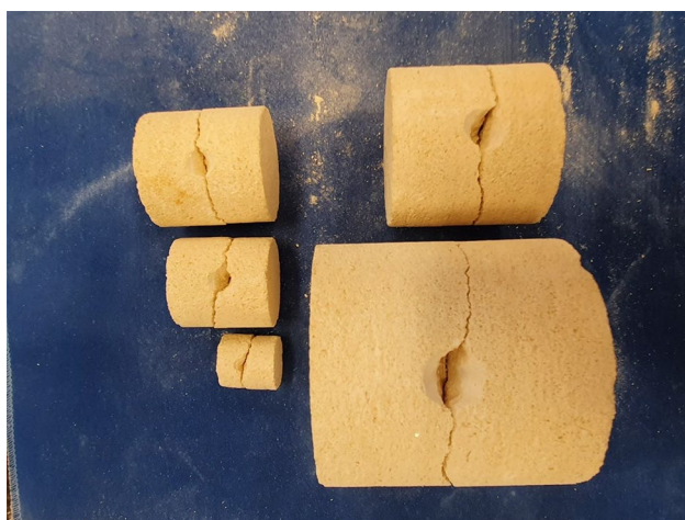
Fig. 19 Typical failure patterns observed from the diametral point load tests on Gambier limestone
