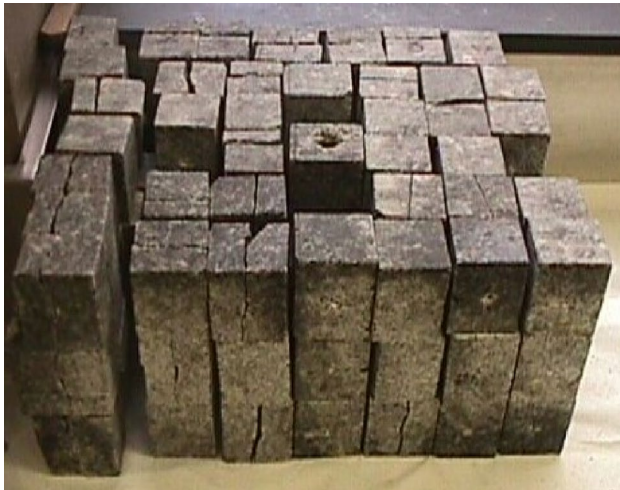
Fig. 12 Division of blasted block in smaller sub blocks (Kunzel 2003)
