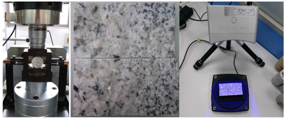
Fig. 1 The granite sample with a single fracture prefabricated by the Brazilian splitting test
