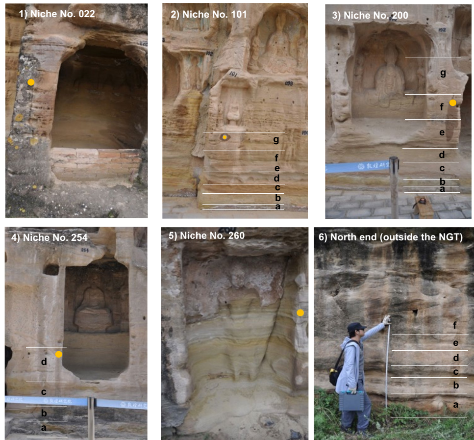
Fig. 2 Images of the six measurement sites on the façade of NGT and the adjacent natural rock outcrop. The letters in 2), 3), 4), 6) stand for layers of beds from which surface hardness were measured. The yellow circles in 1)–5) show the Karsten tube measurement locations
