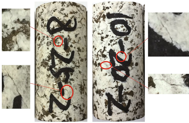
Fig. 1 Cracks formed on the rock specimens after high-temperature treatment at 800 °C and 1000 °C
