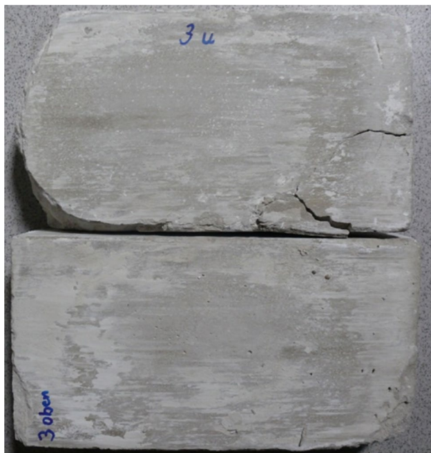
Fig. 9 Typical damage pattern of the sample after the shear test
