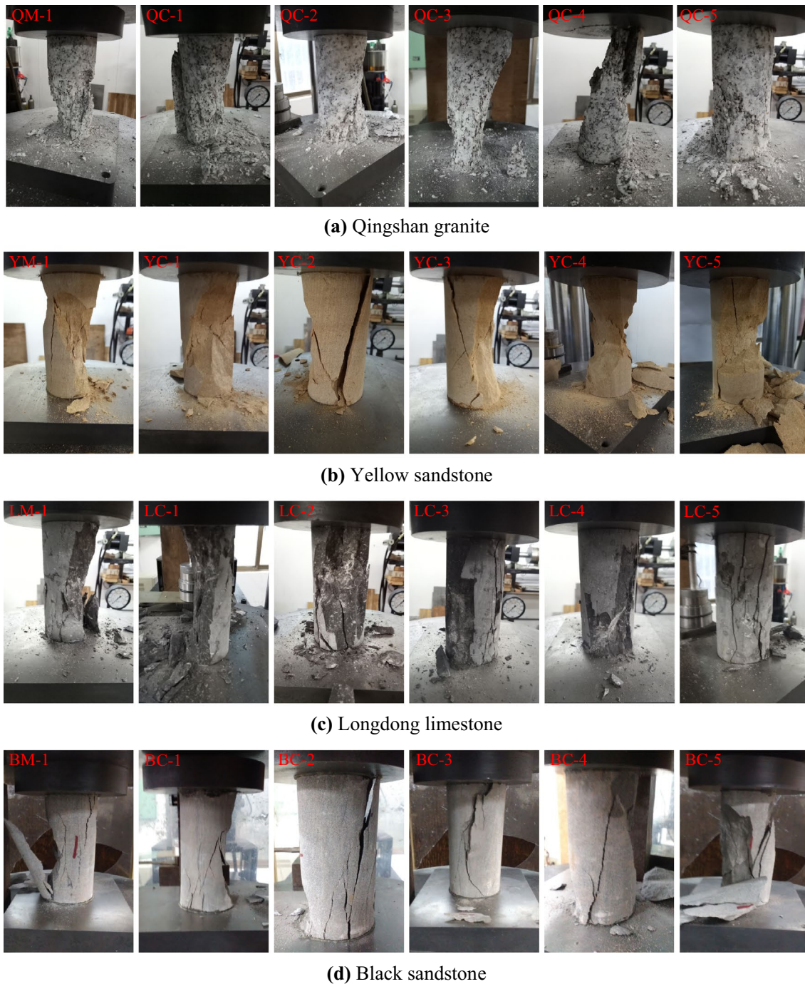
Fig. 6 Failure models of four rocks after UC and SCLUC tests
