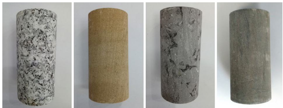
Fig. 1 Photographs of rock specimens (left to right): Qingshan granite, Yellow sandstone, Longdong limestone, Black sandstone (color figure online)
