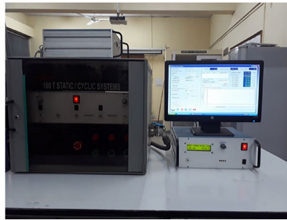
Fig. 1 Schematic and picture of cyclic compression loading frame at IIT Delhi. Input: sinusoidal compression loading output: load and deformation with time
