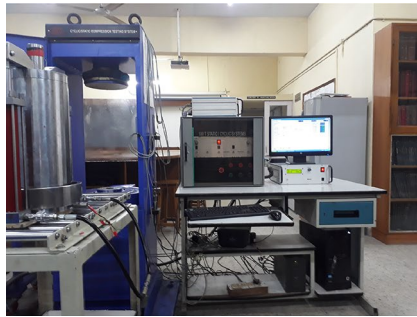
Fig. 1 Schematic and picture of cyclic compression loading frame at IIT Delhi. Input: sinusoidal compression loading output: load and deformation with time
