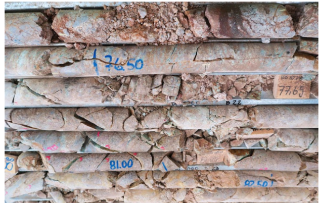
Fig. 3 Cores from a gold-rich porphyry deposit with significant variability
