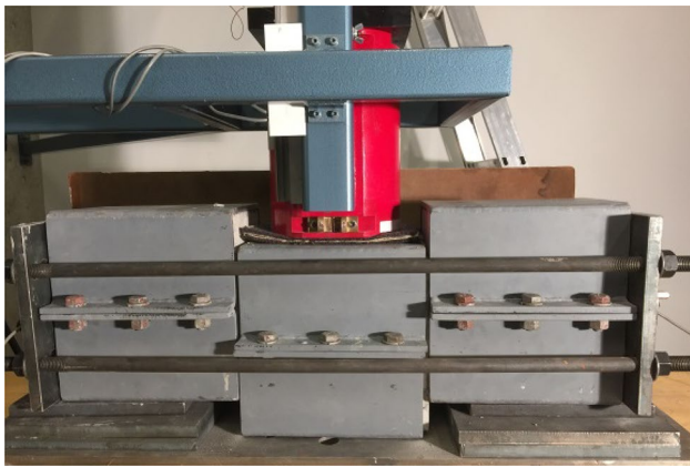
Fig. 13 Failed reinforced DST system after impact
