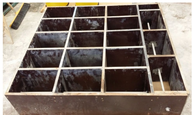
Fig. 3 The plywood moulds used for the sample casting
