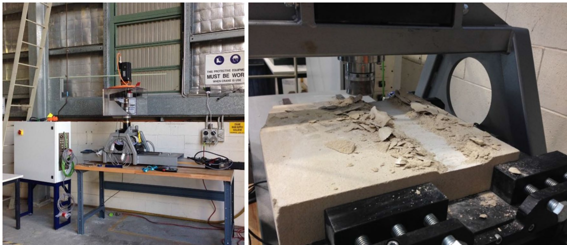
Fig. 4 Overview of actuated disc cutting test-unit, Wobble
