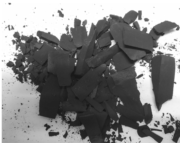
Fig. 15 The peeled sheets of shale after compressive loading
