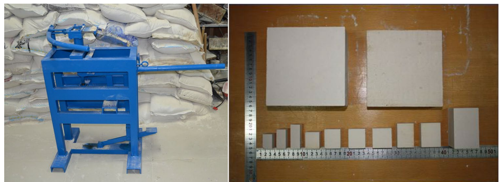
Fig. 6 The tailor-made compressing equipment and various small blocks
