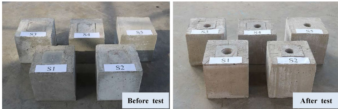
Fig. 2 A layered rock mass specimen before and after a digital drilling test
