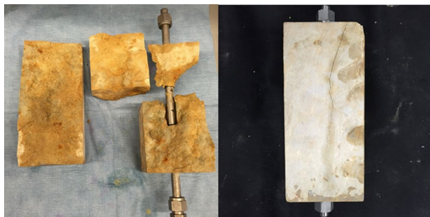
Fig. 8 The 7.5×7.5×15 cm specimens after fracture initiation by HCl (left) and water (right)
