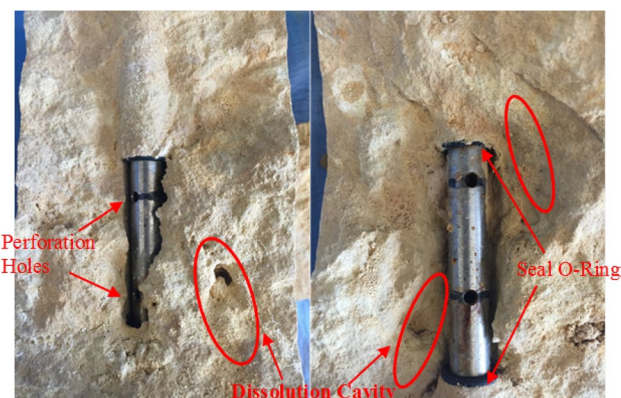
Fig. 9 Dissolution cavities created at 500 psi (left) and 1100 psi (right) target pressures
