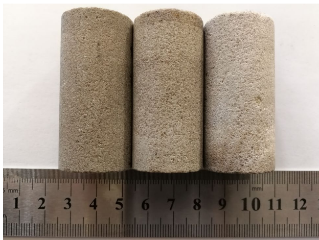
Fig. 1 Typical sandstone specimens from the Silurian formation of Tarim Basin in northwestern China
