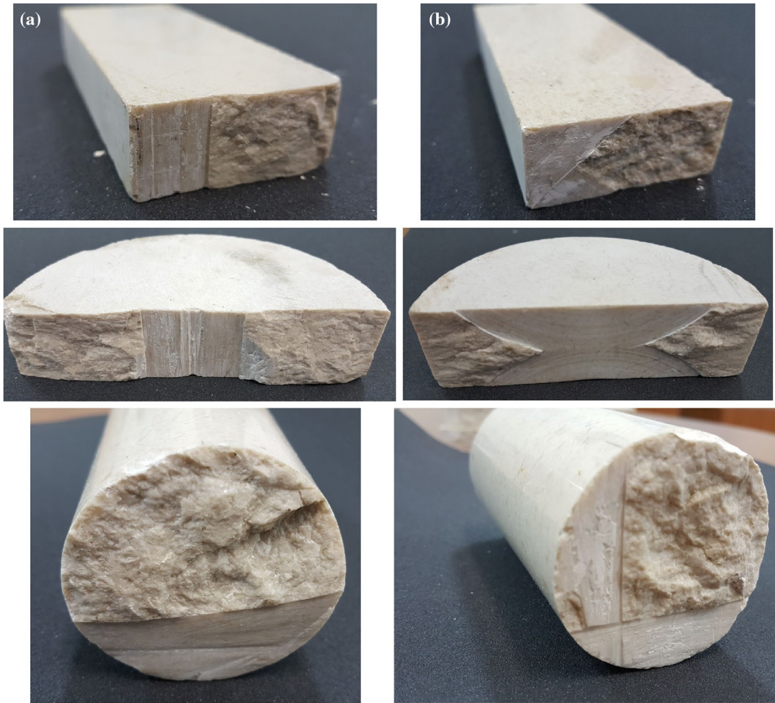
Fig. 8 Fracture pattern observed for the a straight cracked specimens and b chevron notched specimens
