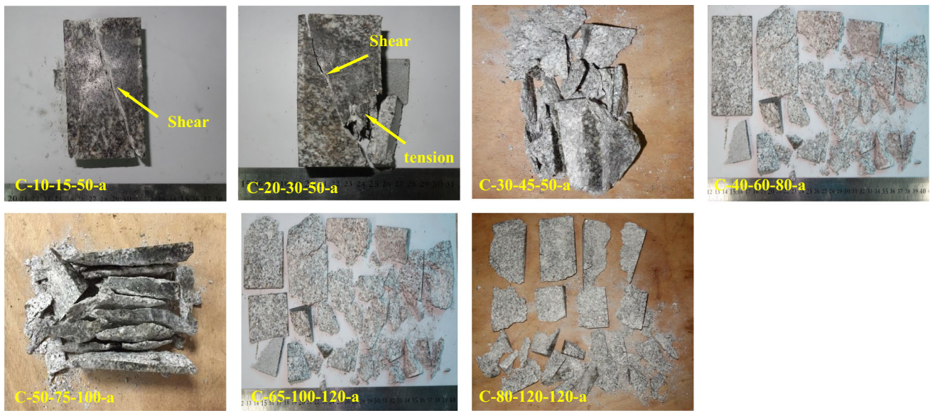
Fig. 5 Failure modes of specimens in true-triaxial unloading test in Group C with \sigma_2/\sigma_3 being 1.5. Note: failure modes of group b are not presented because of similarity and limited space
