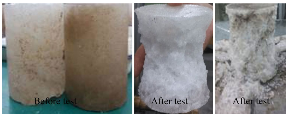
Fig. 1 Specimens before and after the cyclic loading test
