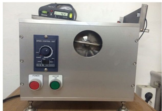
Fig. 10 Photograph of the automated tilt test apparatus used in this study
