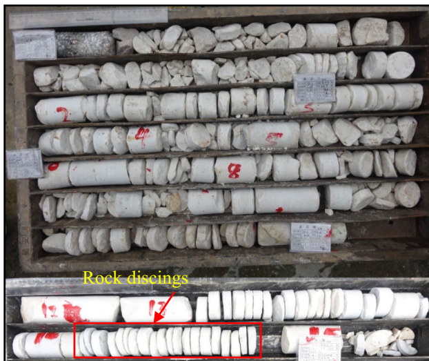
Fig. 4 Rock discing at borehole T8-2 in the south-western sidewall of 8# Lab, at chainage 0 + 045
