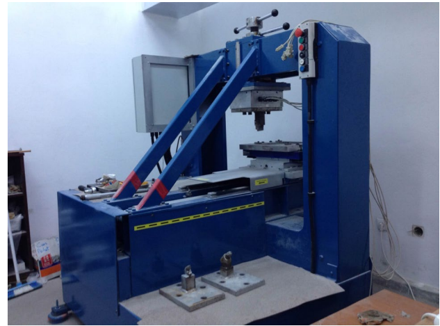
Fig. 6 A photograph of the portable linear rock cutting machine. (Reproduced with permission from Balci et al. 2015)
