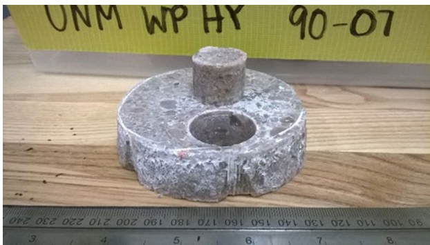
Fig. 2 A 25.4-mm-diameter core obtained from 100-mm-diameter, 25-mm-thick disc of consolidated salt
