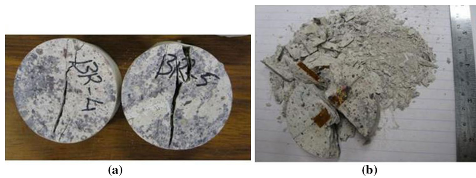
Fig. 10 Brazilian disc specimens of Brisbane tuff after failure, from Erarslan et al. (2014), a monotonic loading, b cyclic loading
