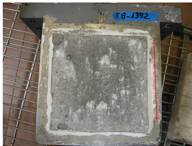
Fig. 10 Concrete surface of sample T8 after the test—the arrow indicates the shear direction
