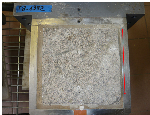
Fig. 11 Rock surface of sample T8 after the test—the arrow indicates the shear direction
