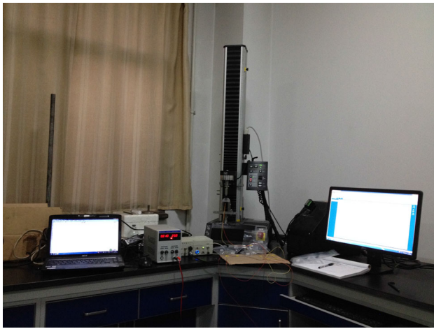
Fig. 4 Experimental setup system for the SCB test
