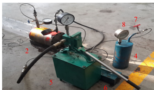
Fig. 2 Experimental equipment for the simulation of coal and gas outburst. a Principle diagram of experimental equipment for the simulation of coal and gas outburst, b apparent of the simulation of coal and gas outburst. 1 The coal sample; 2 simulation system of coal and gas outburst; 3 free weak surface of the outburst outlet; 4 CH 4 gas bottle; 5 axial stress loading equipment; 6 confining stress loading equipment; 7 regulating valve; 8 pressure gauge; 9 liquid medium; 10 acoustic emission testing system; 11 spherical seat; 12 load cylinder; 13 rubber case
