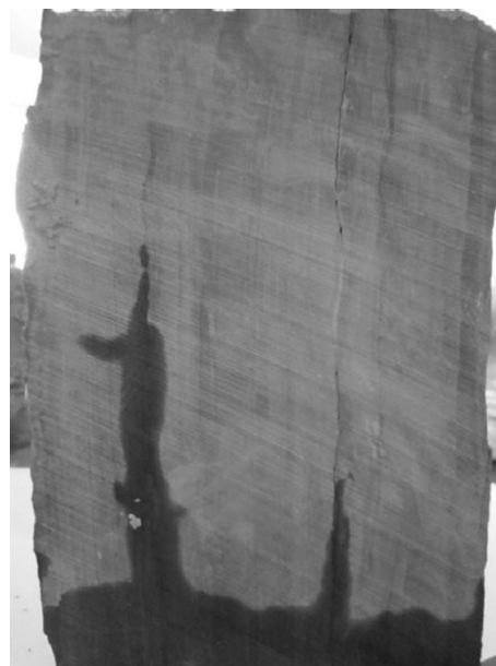
Fig. 14 Capillary self-absorbing phenomenon of shale
