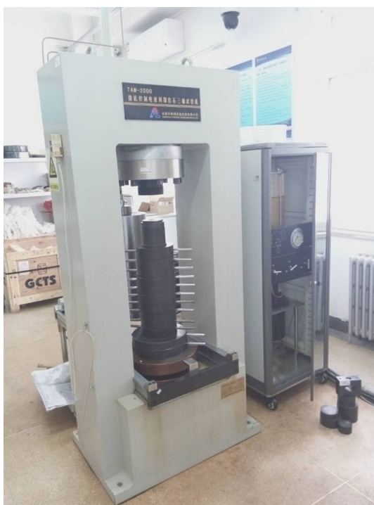
Fig. 1 Photograph showing the TAW-2000 servo-controlled testing system
