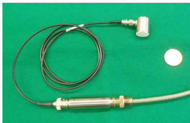
Fig. 3 Typical AE sensor and preamplifier for a laboratory experiment. Coin is 24.26 mm in diameter (a quarter of US dollar) for scale
