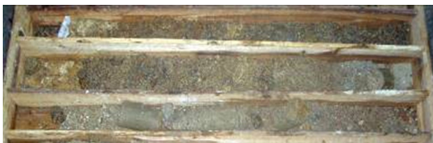
Fig. 8 Sandy soil samples from Sta. YK8+375 to YK8+415
