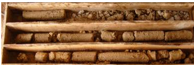
Fig. 7 Silty and clayey soil samples from Sta. YK8+330 to YK8+375
