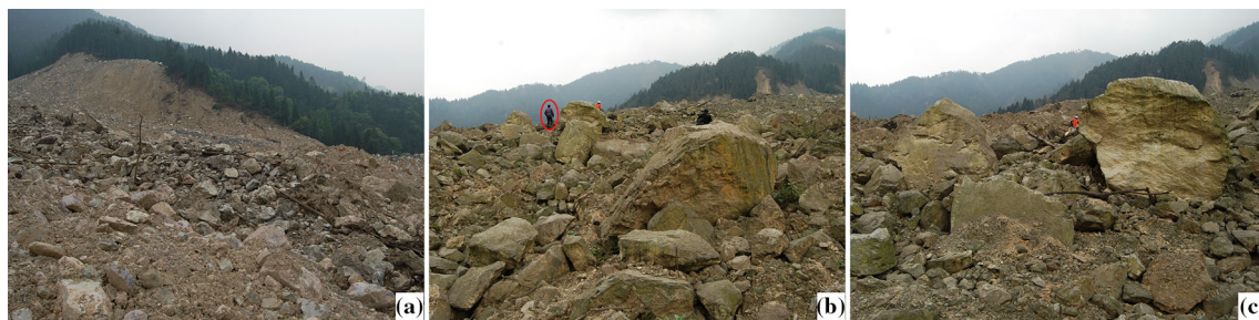
Fig. 6 Display of coarse-grained material deposited on the surface of the Xiejadianzi rock avalanche
