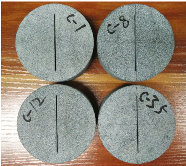
Fig. 2 Virgin CCNBD samples of Dazhou sandstone
