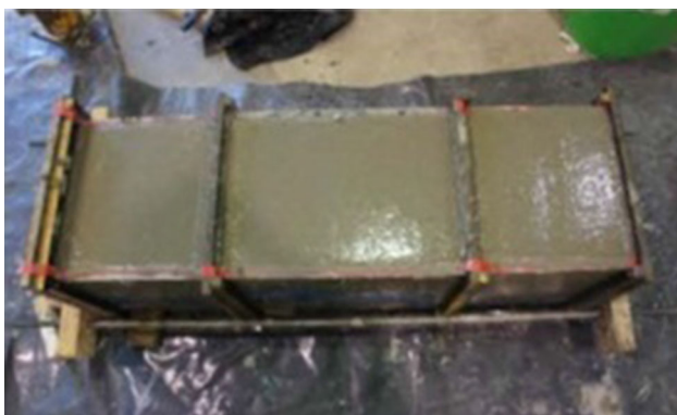
Fig. 5 Concrete block casting
