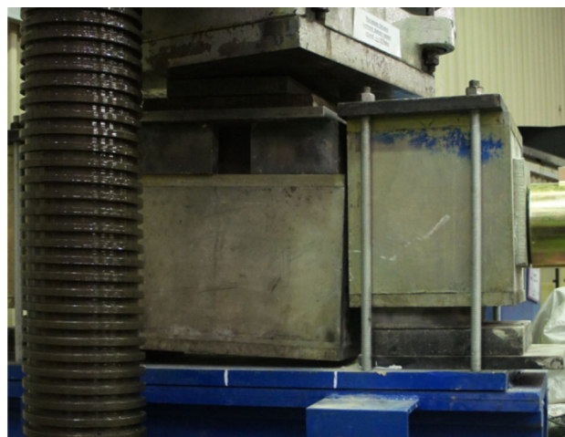
Fig. 6 Sheared central block of the tested cable bolt
