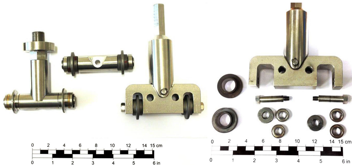
Fig. 6 Tool versions used during the development of the Rolling Indentation Abrasion Test (RIAT) method. From left (initial) to right (current)
