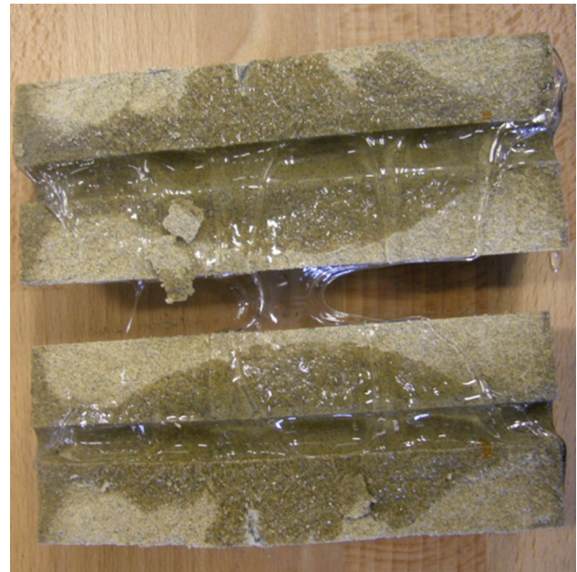
Fig. 12 Hydraulic fracturing of rocks using viscous silicon fluid: the high viscous silicon fluid entered inside the sample through the fractured surface
