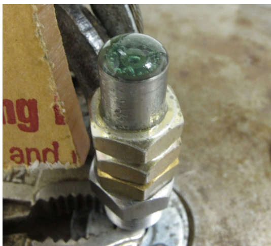
Fig. 6 Brine exiting the pore pressure port at 250 °C
