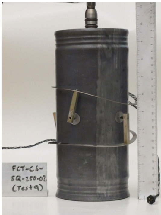
Fig. 2 Instrumented pretest specimen assembly
