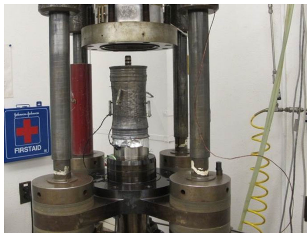
Fig. 3 Test apparatus with reconsolidated sample
